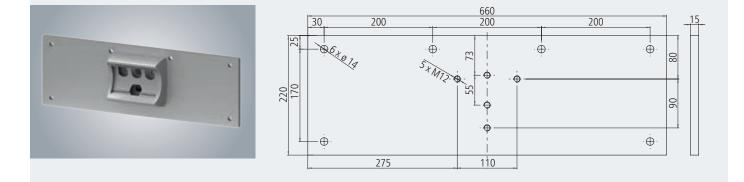
Mounting plate, 660 x 390 x 15 mm + standard wall bracket
